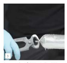
Remove the KÖSTER KB-Flex 200 tubular bag from the warm water (maximum +40 °C) and cut off the front clip of the tubular bag.
