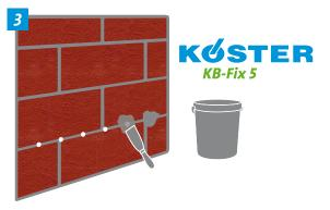
The holes can be sealed immediately with KÖSTER KB Fix 5 flush with the wall surface.
